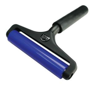
5. Holding the sticky paper with your free hand, clean the silicone roller on the sticky paper by rolling the roller back and forth once or twice on the sticky paper. If the sticky paper has been used multiple times and looks dirty, use a new piece of sticky paper. Note: Wash the silicone roller in warm soapy water if the roller is no longer tacky. Replace the silicone roller if the tackiness does not return.
